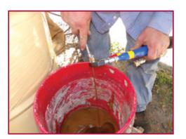
Move the hose to the bucket that is lined with the trash bag and open the valve on the end of the hose. Allow the material to empty into the bag until pure poly is no longer coming from the hose and turn off the valve.
