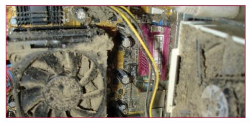
is intended to cool the circuit boards down - if this fan becomes blocked or is not operating properly it will not be able to cool the boards. Following are some simple preventative measures:
