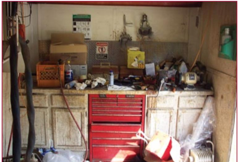
rebuild or clean a gun? Look around the floor at all the debris piled up to the point where you can't even open the cabinet doors. The APR respirators are just hanging on the wall and not in sealed bags stored properly. There is an eye wash bottle on the wall but it is only half full.
