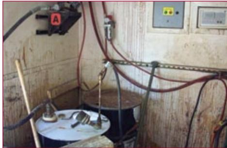
gray handled boat oar which is used to stir the "B" side material, which requires taking the lid off the drum and potentially allowing more debris into the system. These types of practices are harmful to filters and high pressure seals and to the overall performance of the equipment.
