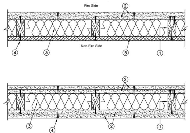
1. Wood Studs — Nom 2 by 4 in., spaced 16 in. OC, effectively braced and firestopped at top and bottom.
