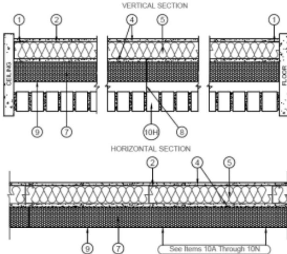
1. **Steel Floor and Ceiling Tracks** — Top and bottom tracks of wall assemblies shall consist of steel members, min No. 20 MSG (0.0329 in., min bare metal thickness) steel or min No. 20 GSG (0.036 in. thick) galv steel or No. 20 MSG (0.033 in. thick) primed steel, that provide a sound structural connection between steel studs, and to adjacent assemblies such as a floor, ceiling, and/or other walls. Attached to floor and ceiling assemblies with steel fasteners spaced not greater than 24 in. O.C.
