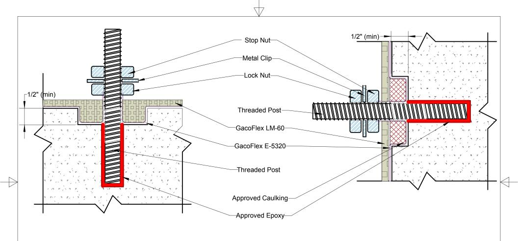
If a vapor barrier is required, it must be applied prior to the bolt installation.
